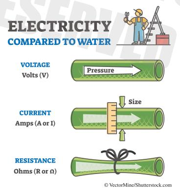
Remove the kink and water goes back to flowing as before. Same in an electrical circuit. If there is an unwanted increase of resistance, the current is reduced. I hate to do this to you, but let me show you.
