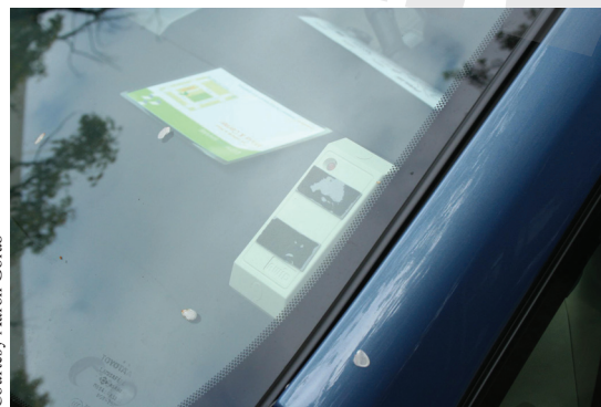
The windshield-located card reader on a car-share vehicle in Berkeley, California.
